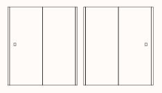
Panel: 600/900mmW Floor Height: 1050mm Depth from left/right side: 100mm External Swing door left or right side Switch can be placed on left hand or right hand front panel
